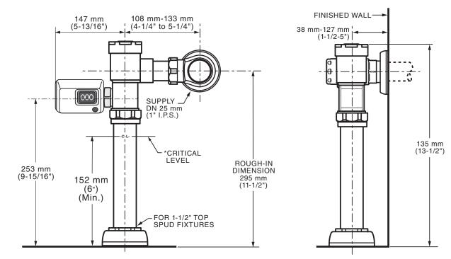
\*Note: The Critical Line (-C-L-) on Vacuum Breaker must typically be 6" (152mm) minimum above fixture. Consult Codes for details.
